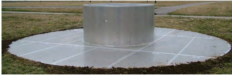
Figure 39. Photo of top hat calibration target from Gotcha data set. [25].
